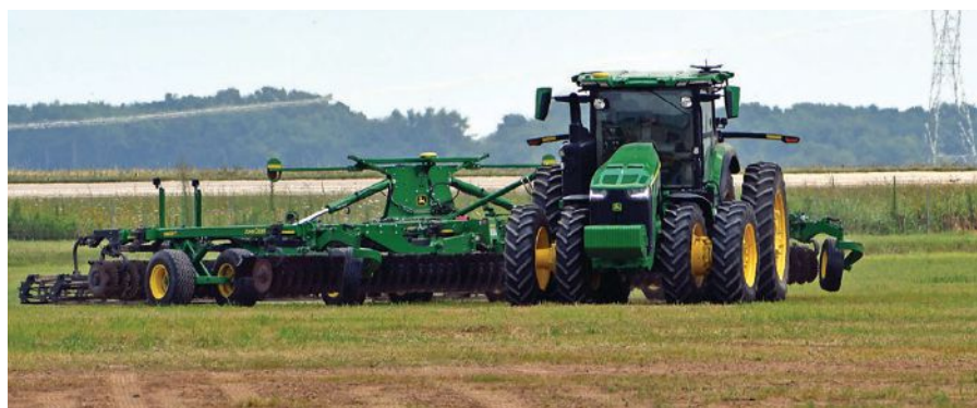
FOLLOWING THE PATH: The autonomous tractor follows the path laid out in the Operations Center. It turns by itself and can stop on a dime.
